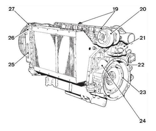
19 The transport device 20 Turbocharger working on exhaust 21 Speed controller 22 Housing SAE22 23 Flywheel 24 Starter 25 Coolant level 26 Air valve 27 Cap for coolant
